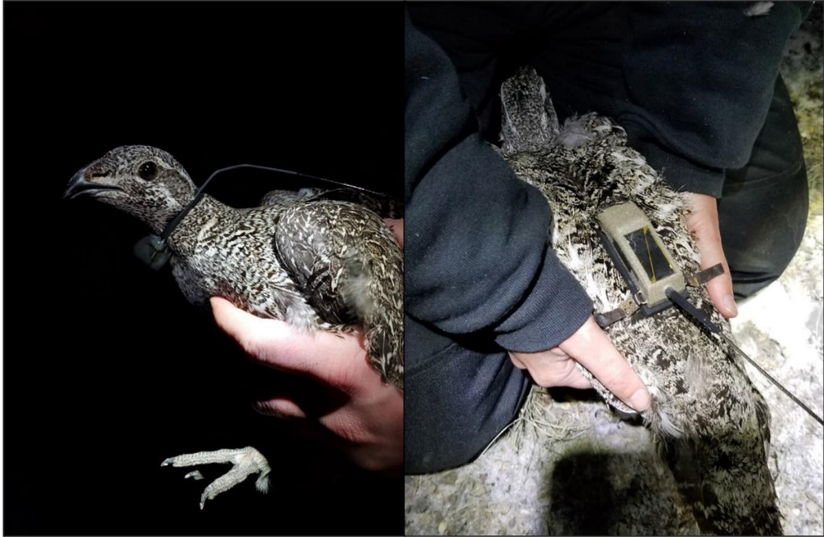
Figure 8.22. Photos showing the necklace-style very high frequency (VHF) collar (left) and backpack-style global positioning systems (GPS) transmitters (right) attached to female greater sage-grouse in the Pahsimeroi Valley of Idaho, USA (Stevens et al. 2023).
